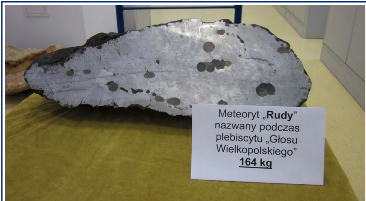
Figure 9. One of the biggest chunks (164 kg) of meteorite Morasko, exposed in museum of Faculty of Geographical and Geological Sciences of Adam Mickiewicz University in Poznań. This coarse-grain octahedrite (Muszyński et al. 2012) contains also rounded black nodules composed mainly of graphite and various trace compounds. Among the latter are also two new minerals discovered in the Morasko meteorite: moraskoite (Karwowski et al. 2015 ) and czochralskiite (Karwowski et al. 2016).
